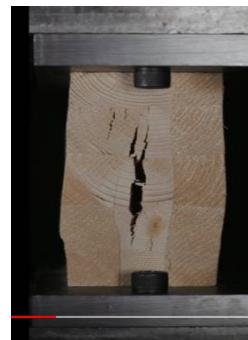
Compressive failure of a timber block
