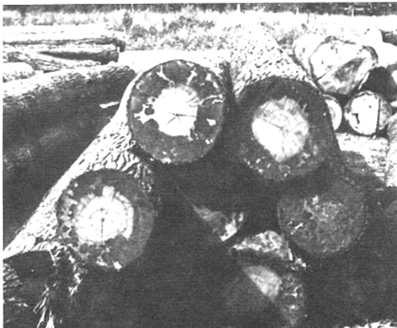
Logs with heavy sapwood stain at the ends.
