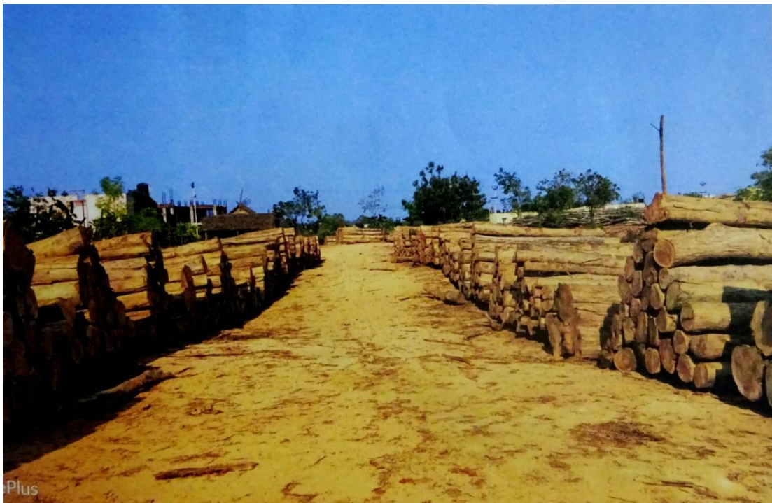
Stacks of lots with sufficient aisle space for movement of vehicles
